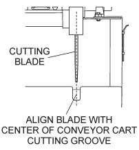
Figure 28. Cutting Head Alignment (Horizontal)
